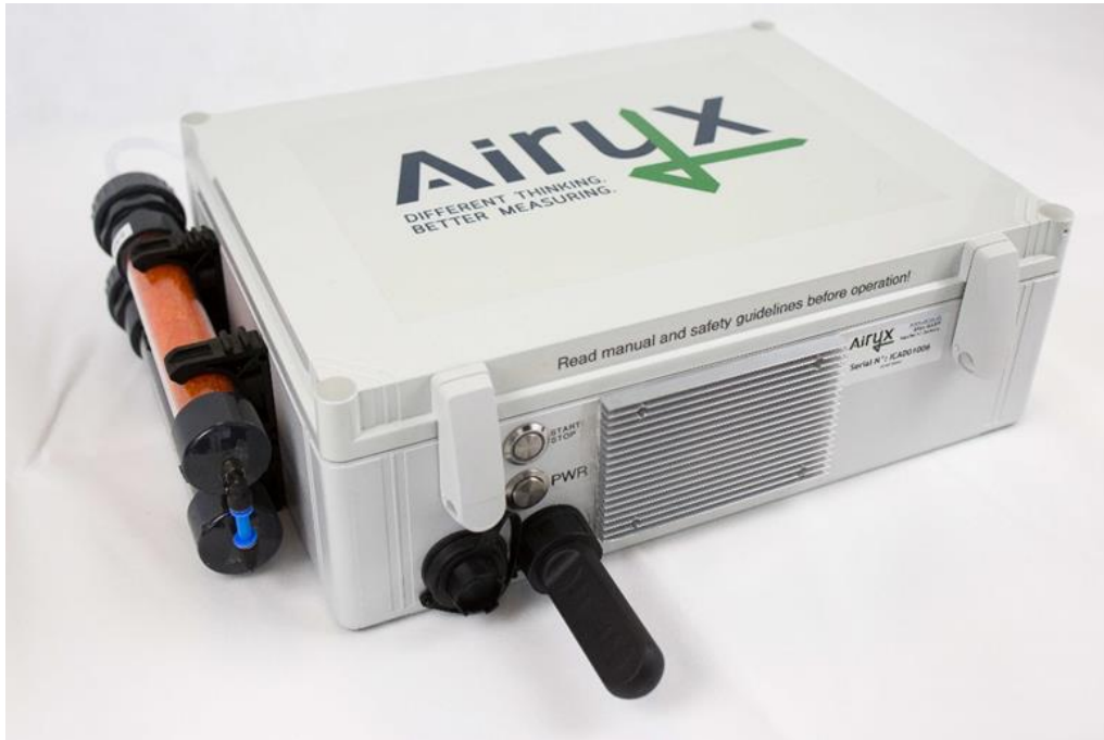
Figure 17 Airyx ICAD NO 2 /NO x /NO Monitor [20]. This instrument model was used for the plume chasing
