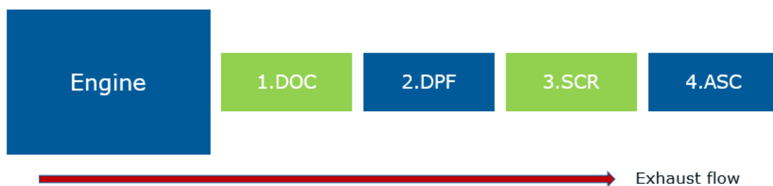
Figure 2 Schematic drawing of an exhaust aftertreatment system (EATS) setup and the arrangement of the single components in the exhaust stream
